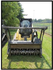
Caterpillar skid-steer with a Fecon™ mounted mulching head used to clear understory bush honeysuckle from UI experimental forest.
